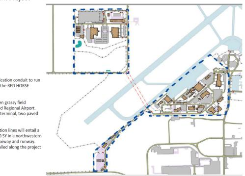
Installation of a new communication conduit to run from the Cantonment area to the RED HORSE Enclave.
